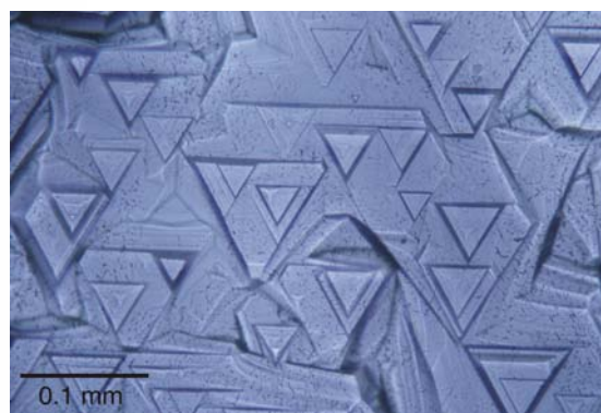
Figure 3. Surface with trigons and micro-inclusions at 15 µm beneath the diamond surface.
